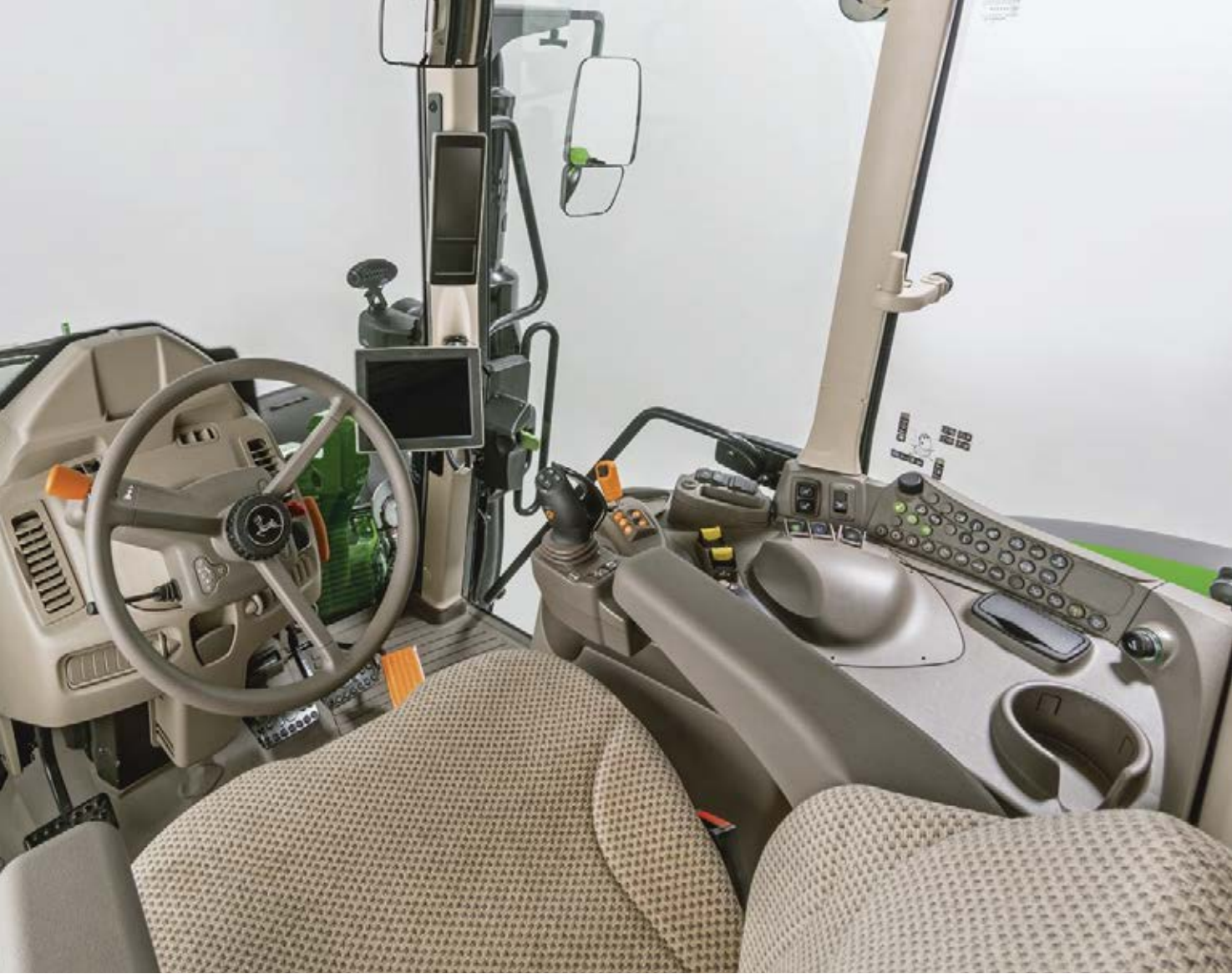
Intuitive, streamlined tractor function control at its finest: The Corner Post Display in A-post and the right-hand console.
